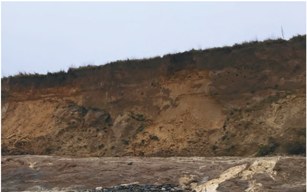
Figure 3. Happisburgh Glacigenic deposits exposed in the cliffs at the north-western end of the site. The cliffs are formed in mostly silty SAND, the base of the cliffs and foreground is slightly sandy slightly gravelly CLAY.
